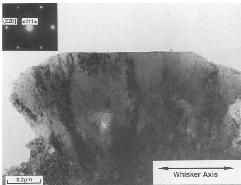
Figure 3 Electron-transparent region of TiN whisker, its \langle 111 \rangle zone axis is aligned with the electron optical axis. The inset shows an electron diffraction pattern comprised of (220) reflections.
